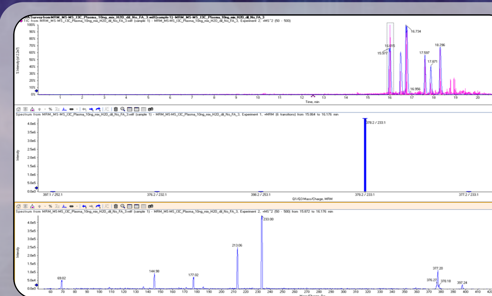
Figure 4. Example result from LC-MS/MS: 10ng mix of all compounds after dilution with water, extraction from plasma, and reconstituted with mobile phase, run on an MRM-MS/MS scan. The first peak is at 16 minutes, showing that this compound was first to leave the LC column. The blue trace shows the MRM result, and the pink trace shows data-dependent transition from MS/MS scan. An MRM scan is 'multiple reaction monitoring', and is used to detect only ions which produce a specific fragment. MRM peaks can be highlighted to identify specific ion transitions. The bottom trace shows the mass spectrum (fragmentation pattern) of this compound.
